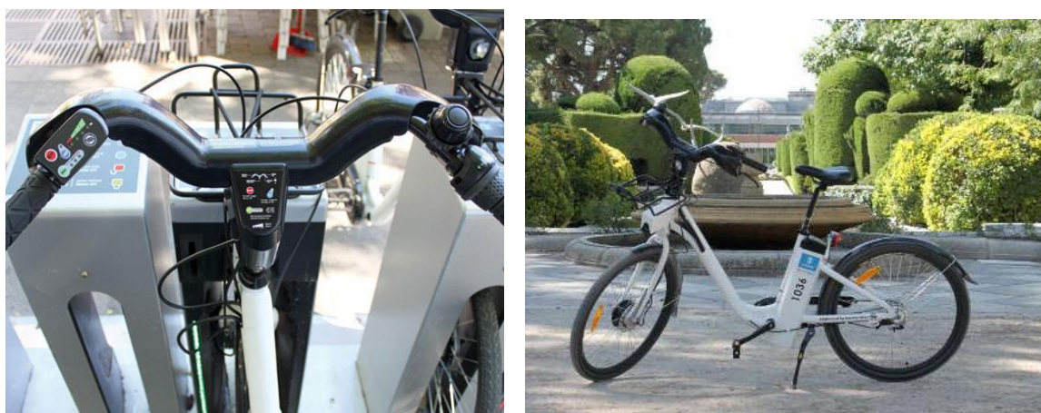
Figure 25. Fork lock dock station of Madrid electric bike sharing system
