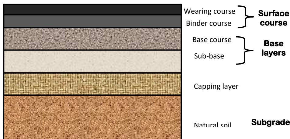
Figure 12. Composition of a pavement structure
